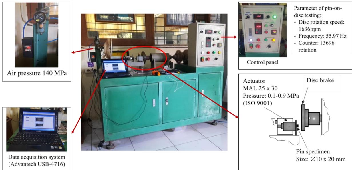
**Figure 2. Schematic pin-on-disc testing**
