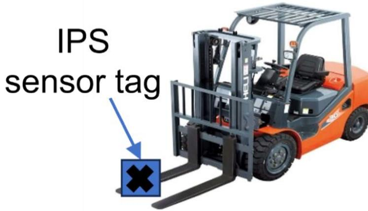
Figure 4. Sensor placed on the forklift
