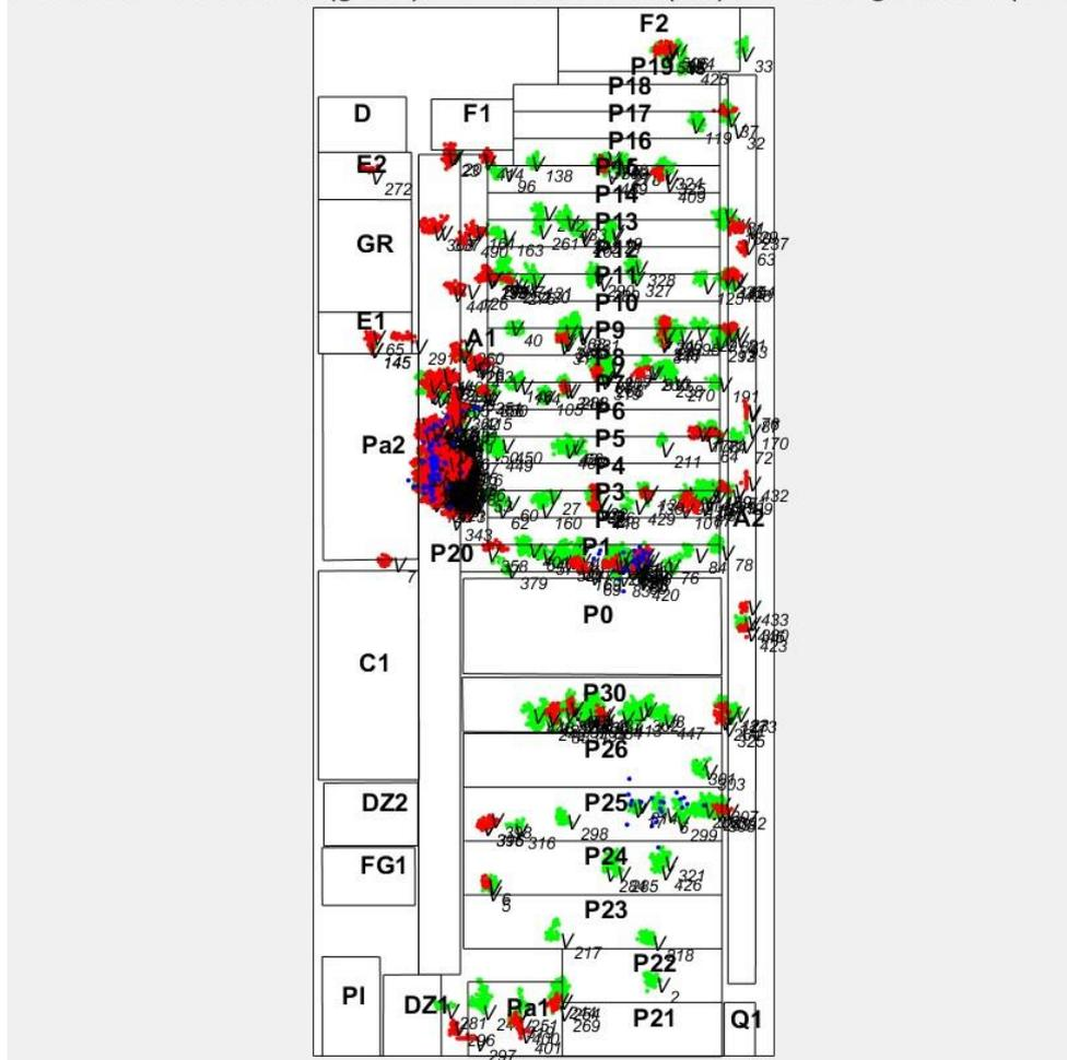
**Figure 10.** With the modified DBSCAN algorithm, the position data-based clusters can be classified and differentiated based on forklift fork movements, enabling the identification of distinct value-added, non-value-added, and waiting activities
