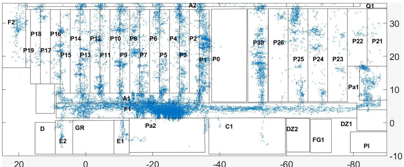
Figure 5. Indoor positioning data-based movement of forklift in a warehouse environment. Sufficiently accurate location data is important for identifying the logistics area
