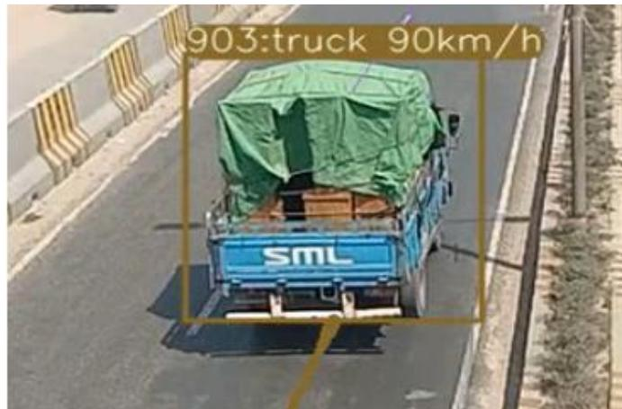
**Figure 7. Speed calculation**
