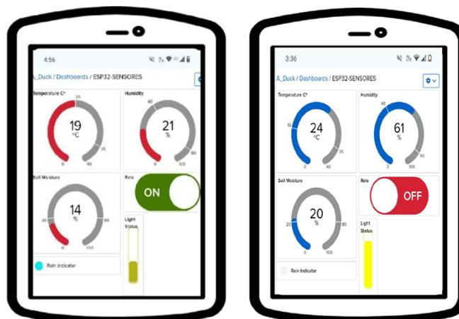
Figure 34. Adafruit IO Interface with Normal Sensor Statesview (left) and Warning modeview (right)
