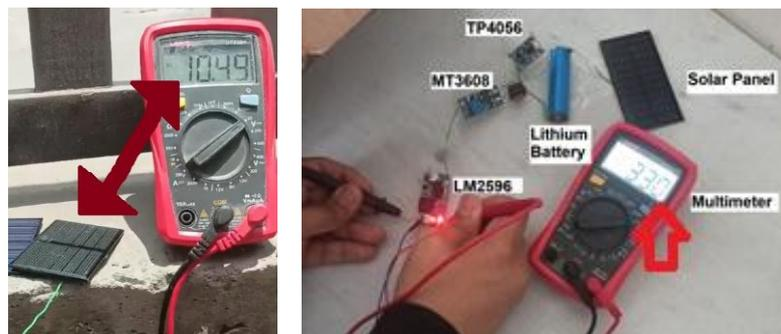
Figure 23. Operation of: Solar Panels view (left), Power System Sensors view (right)
