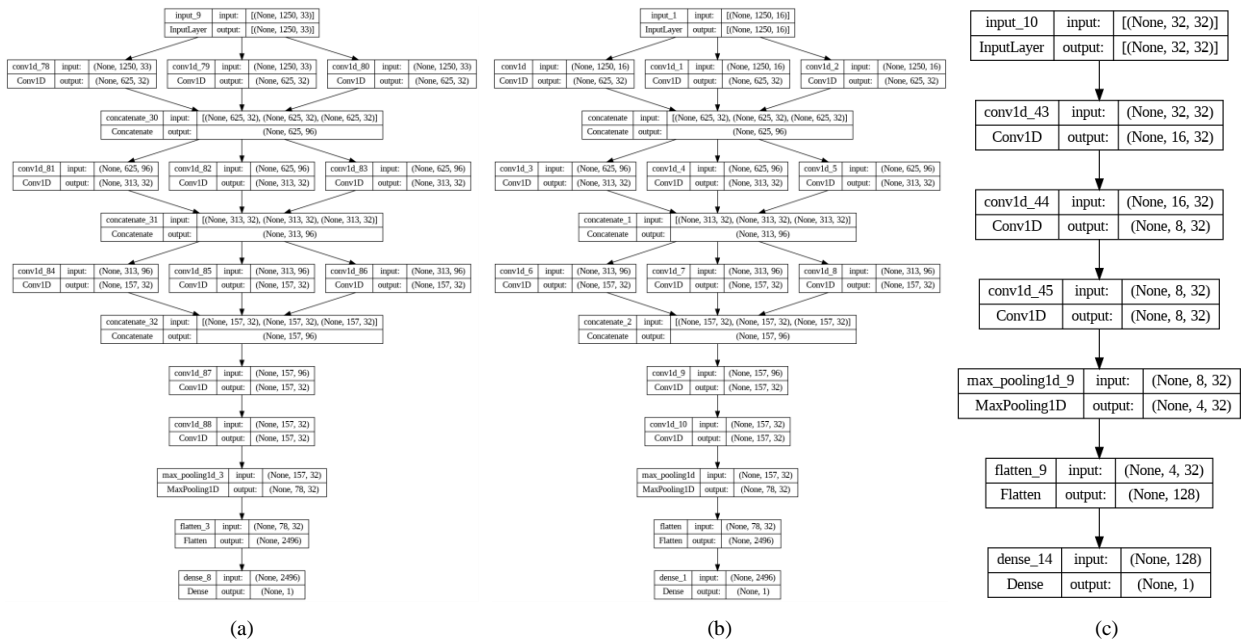
Figure 9. The CNN model architecture for the: (a) first and second experiments; (b) third experiment; (c) fourth experiment
