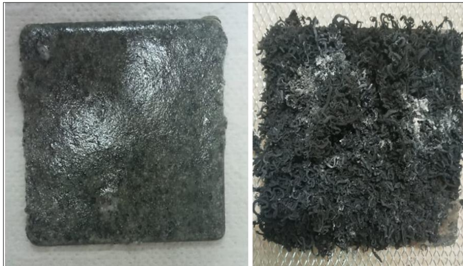
Figure A-4. IF-3 coated samples before and after fire test
